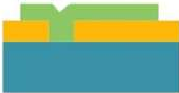
Deposit/pattern structural layer
