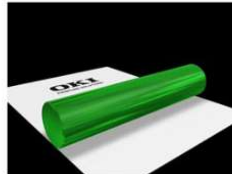
4. Transferring: The image formed of toners on the drum is transferred to paper.
