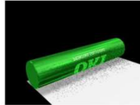
2. Developing: Toners are attached to the latent image formed on the image drum.
